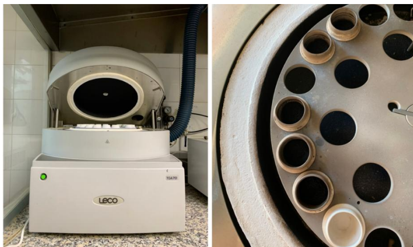
Figure 15 TGA used as a programmable furnace (left) and carousel for samples (right)
