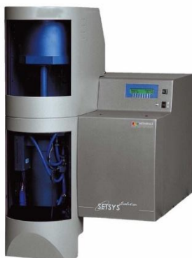
Figure 20 Thermogravimetric analyser for TGA DSC. Source: Setaram Instrumentation official website
