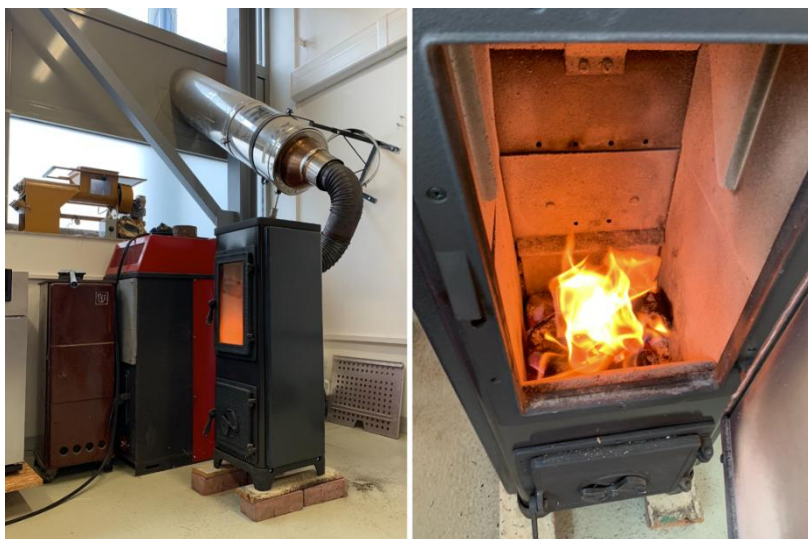
Figure 19 Combustion unit (left) and burning briquettes made from H.mantegazzianum (right)
