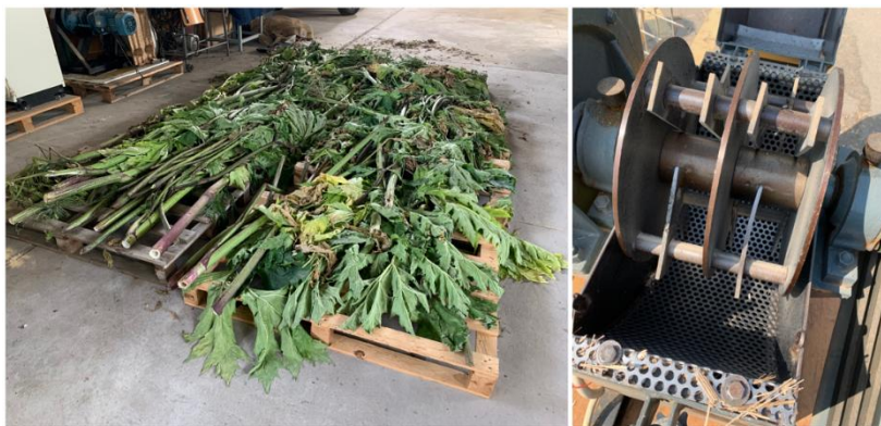
Figure 10 Preliminary drying of summer-harvested biomass (left) and internal view of hammer mill with sieve (right)
