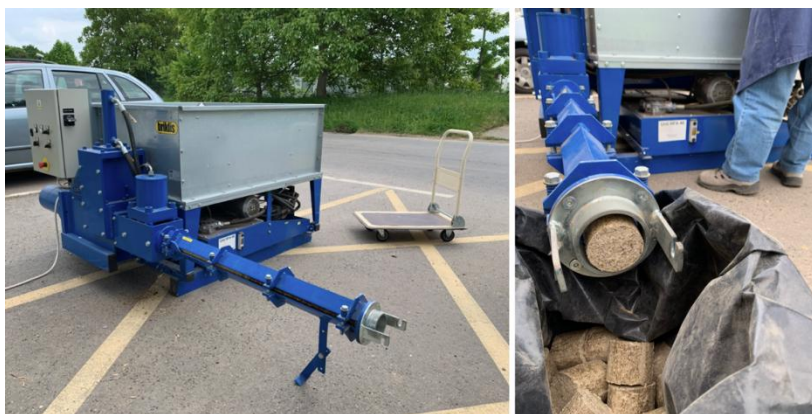
Figure 17 Hydraulic briquetting press (left) and briquetting of material (right)
