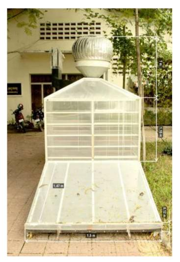
Figure 3.5 Photograph of a natural convection solar dryer
